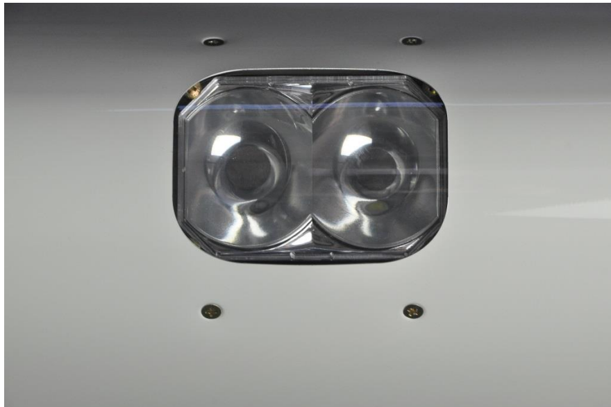
Figure 5-29: LED Landing Light
