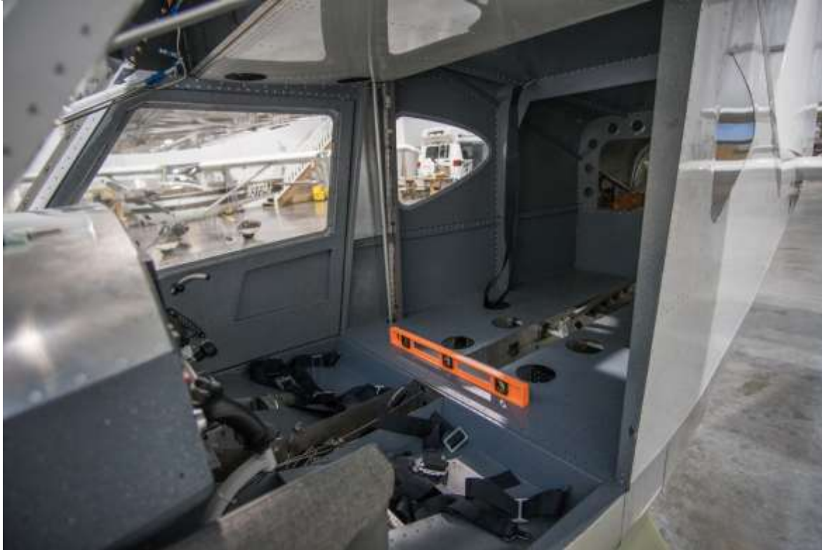
Figure 5.7.24.2 Lateral leveling of the aircraft.
