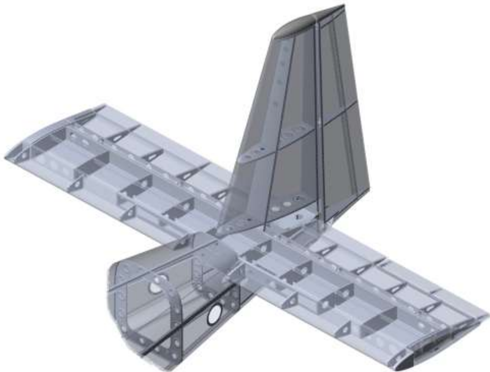
Figure 5.7.5.1 Empennage structure with skin hidden.
