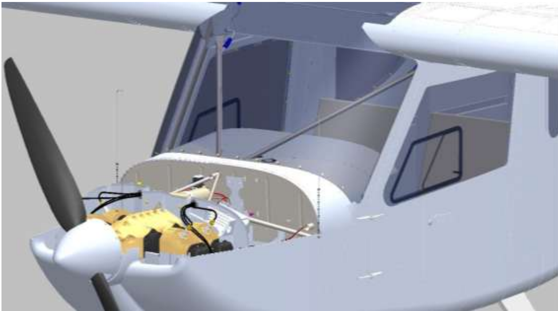
Figure 5.7.9.6 Lower cowl hinge pin removal.
