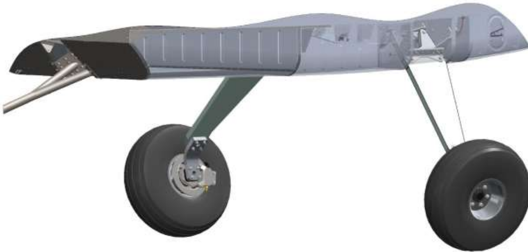
Figure 5.7.7.1 The main landing gears with fuselage skin hidden for clarity.
