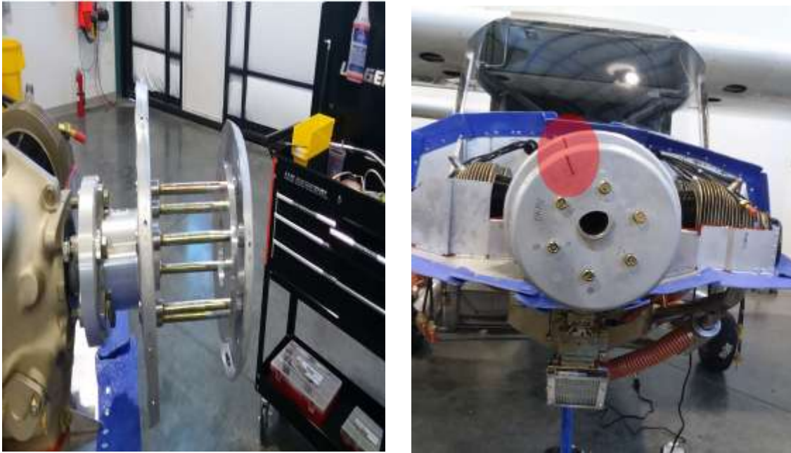
Figure 5.7.16.7 Front spinner bulkhead alignment.
