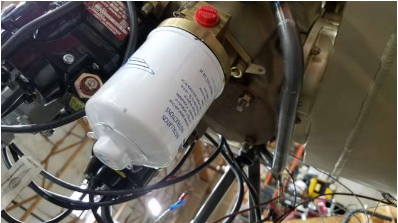
Figure 5.7.10.1 Oil filter secured by safety wire.
