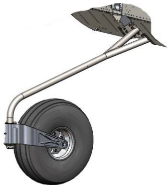
Nose landing gear (fuselage skin hidden for clarity)
